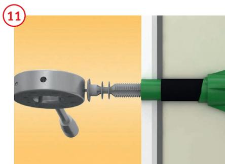
Then the screw channel is sealed with the **rocketseal** plug, screwed using the **rocketkey** Allen assembly key and camouflaged with a 'dab' of façade paint. Generally, we do not use acrylate or other sealing agents at this point because they often leave marks on the façade later. The design of the plugs guarantees the required tightness and is simply screwed in.
