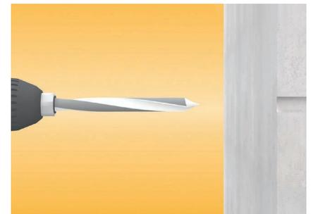
Pre-drill the borehole with a **drill (diameter 14 mm)** to a depth of 120 mm and blow out the borehole.
