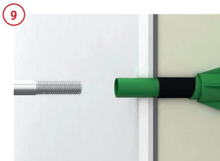
Then the **rocketbolt** anchor screw can be unscrewed. (Note: As the **rocketbolt** anchor screw is an important part of the anchor system that the building owner also buys, this screw remains with the customer. We recommend storing this in one or several packages in the heating room so that this can be reused again later or that it can be accessed quickly.
