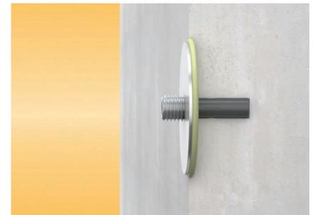
Insert the enclosed plastic wall plug into the borehole. Apply a thick layer of **rocketglue** to the back of the **rocketbase** so that there are no air chambers when the anchor plate is screwed in, the anchor plate has full contact and a bead of excess material oozes out. After wetting the **rocketbase**, screw in the anchor and tighten with the Torx bit from the assembly set using the cordless screwdriver or matching ratchet.
