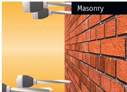
Use the drilling template (card cover in the package) to mark the 4 drilling points, then remove the drilling template again. Pre-drill 4 boreholes with a **drill (diameter 10 mm)** to a depth of 100 -110 mm and blow out the borehole. *(Please always ensure that the wider point of the **rocketbase** is attached horizontally and not upright)*
