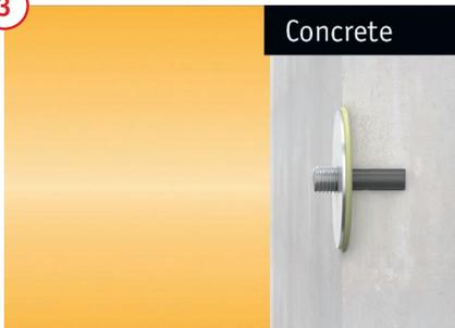
Insert the enclosed heavy-duty metal wall plug into the borehole. Apply a thick layer of **rocket** glue to the rear of the **rocketbase**, so that there are no air chambers when the anchor plate is screwed in, the anchor plate has full contact and a bead of excess material oozes out. After appropriate wetting, screw the **rocketbase** into the metal wall plug and tighten with the Allen **rocketkey**.
